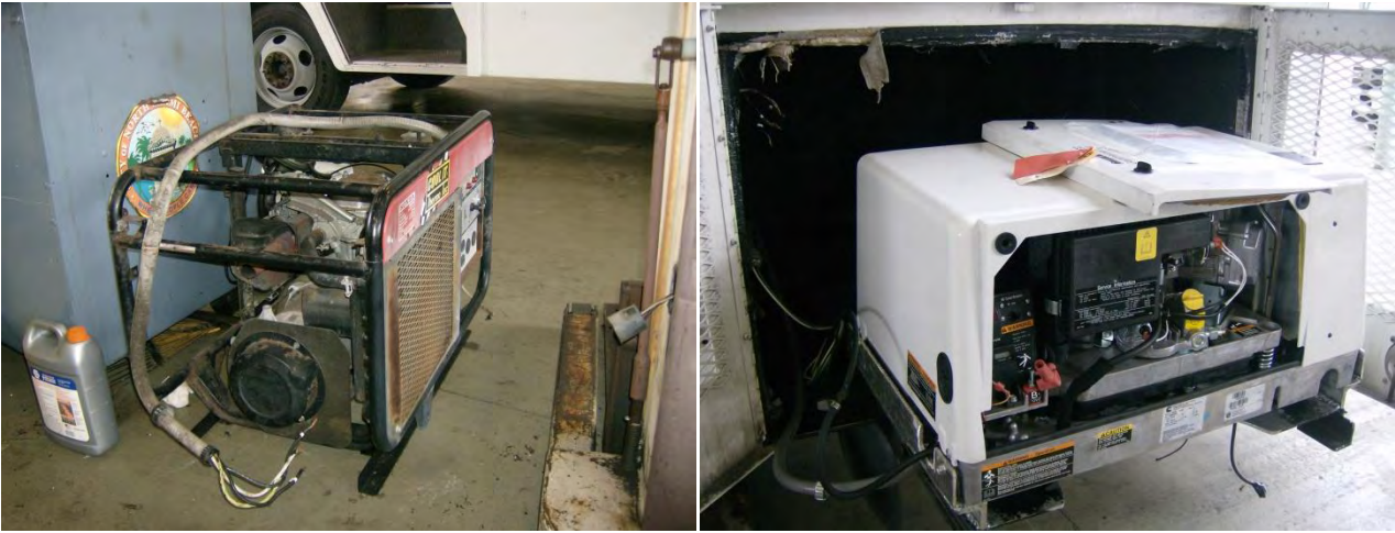
Replaced Auxiliary Power Unit in-house on Mobile Resource Center resulting in savings of approximately $1,200
